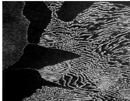
Microstructure of a plain carbon steel that contains 0.44 wt% of carbon
